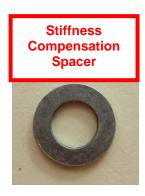
After placing the calibration spacer, jog the platens together until there is less than a 1 mm gap between the upper platen and the spacer. If this gap is too large, the software utility will take a very long time to run. However, do not allow the upper platen and the spacer to come in contact. If the platens are crashed together the load cell will likely be damaged.
