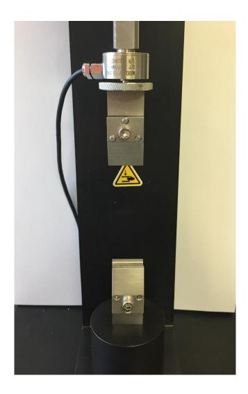
7. A Zero Position Calibration is required after changing grips or platens. See **Section 8** of this manual for more details.
