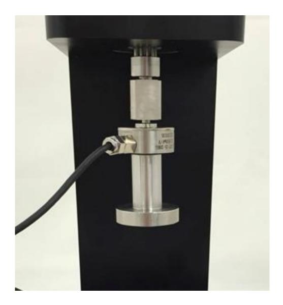
4. Choose an appropriate riser and attach the bottom platen. Use an **M5x14** fastener for a test setup with **NO** riser, a **M5x55** fastener for a 40mm riser, and an **M5x100** fastener for the 80mm riser.
