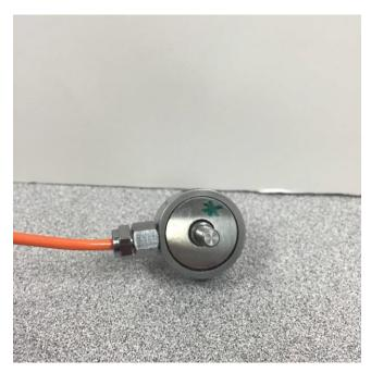
2. Attach the appropriate thumbnut to the **NON-MEASURING END** of the load cell (M5 or M3 depending on the load cell).
