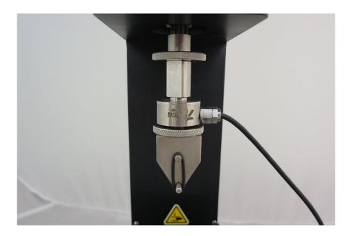
Finger tighten all components. Beware of exerting excessive off-axis and torqueing forces to avoid damage to the load cell.
