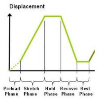
**Holding** - The deformation can be held for a given duration. The duration for which it is held is dependent on the nature of the testing.
