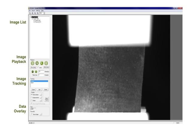
The basic UniVert system comes with a Logitech HD 1080p webcam intended to be used for recording images for image playback and review. This camera and software associated with it **does not** support image tracking.
