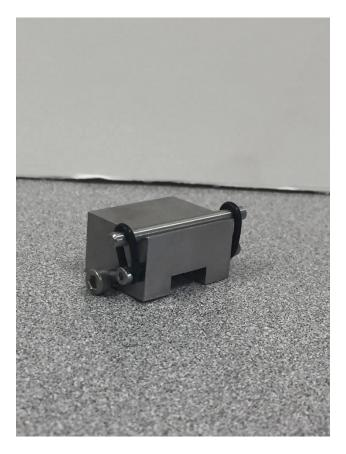
5. Screw the bending block onto the measuring end of the load cell and tighten in the correct position using the locking disc.
