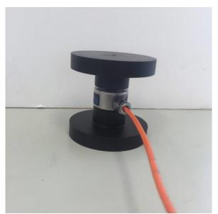
3. Orient the setup such that the measuring end of the load cell is facing up and continue with the standard calibration procedure described above.
