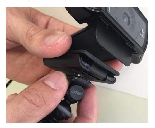
3. Set the camera in the desired recording position using the flexible tripod.
