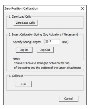
3. Place the provided calibration spring on the bottom platen or grip.
