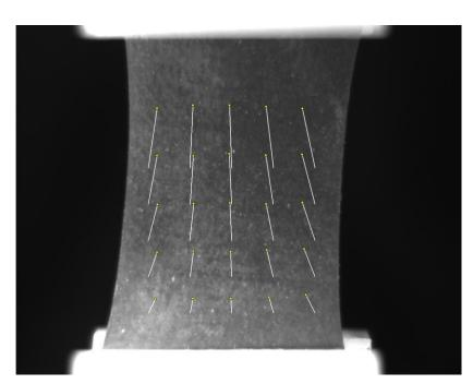
Figure 3: Tracking to 33% strain displayed as displacement.
