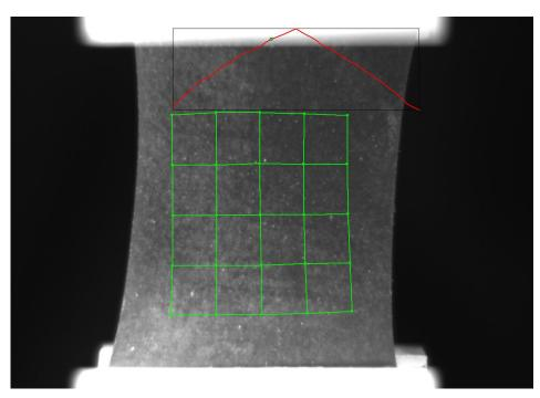
Figure 5: Tracking to 33% strain with overlaid force graph.
