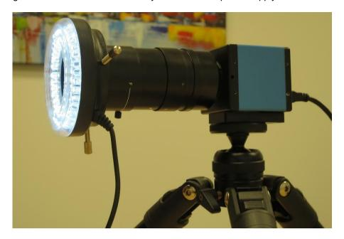
5. Bring the camera to the desired height by adjusting the separation of the tripod legs. Note that working distance from specimen to lens should be at least 15cm.
