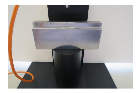
7. Secure both sliders onto the rail in the desired position by tightening the fasteners.
