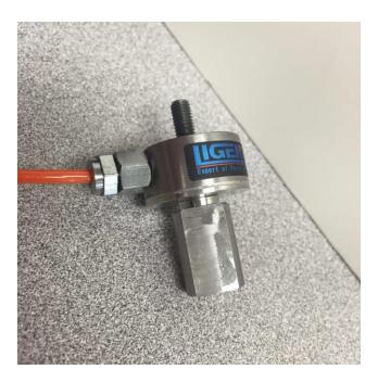
3. Screw the load cell/thumbnut combination onto the actuator. At this point the measuring end of the load cell should be facing down, and the non-measuring end attached to the thumbnut and actuator.
