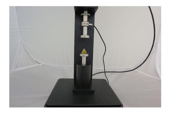
5. A Zero Position Calibration is required after changing grips or platens. See **Section 8** of this manual for more details.
