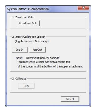
The calibration utility will slowly drive the platens together until the full-scale load is reached on the load cell. Resulting load displacement data is typically very linear and a best-fit slope is used to determine the calibration factor. Compensation is calculated in compression but is assumed to act linearly in both tension and compression. Typical compensation factors are shown in the table below:
