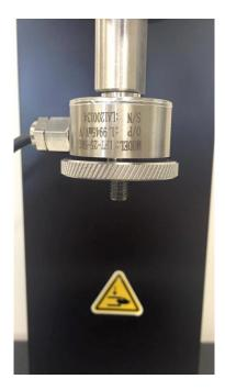
4. Screw the appropriate grip onto the measuring end of the load cell after the locking disc. Tightening the locking disc against the grip allows the grip to be secured to the actuator at any rotational position.
