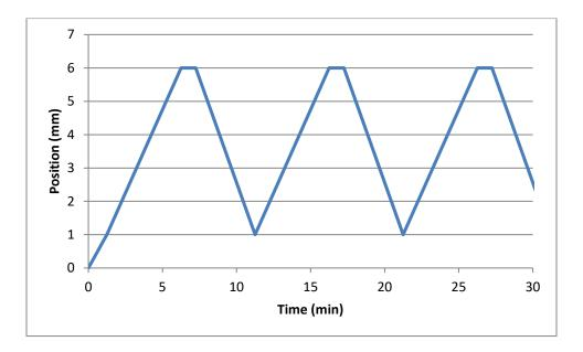
The resulting actuator motion versus time graph for the first 30 minutes:
