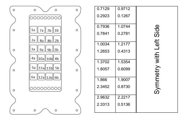
% axial strain, % engineering shear strain per mm of actuator travel with an unmodified well plate.
