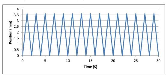
The resulting actuator motion versus time graph for the first 30 seconds:
