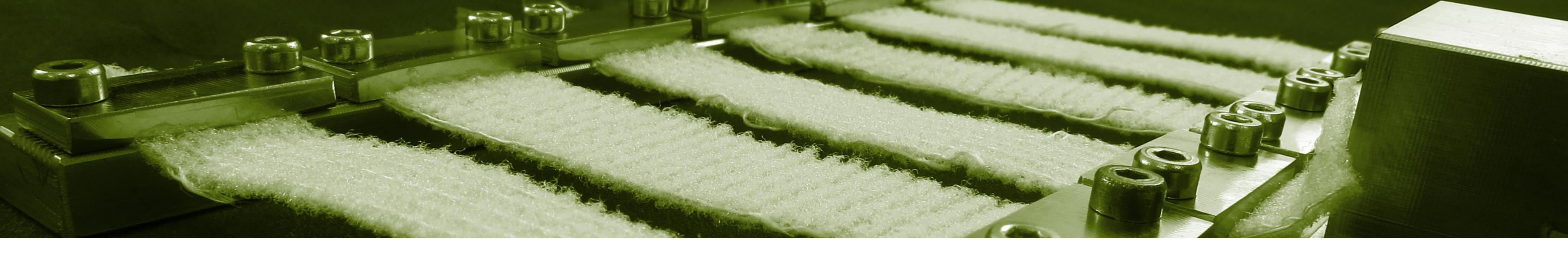
The MechanoCulture T6 can be programmed to run constant velocity or sinusoidal stretch patterns. Magnitudes, frequencies, rest periods, and cycle counts can all be specified in the software application and programmed to the device.
